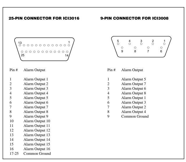
Figure 5. Alarm Pin-Out Configurations
